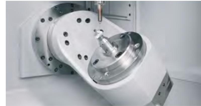
**FZ 08 S five axis:** Integrated 2-axis rotary table (BC kinematics), maintenance-free torque drive technology and automatic tool change with the pick-up method.
