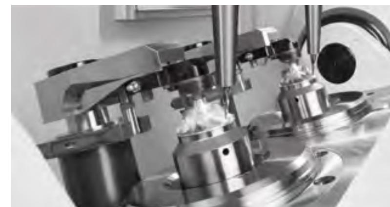
**DZ 08 S five axis:** Double productivity in a small space. The smallest and fastest double-spindle machining center with a 2-axis tilt rotary table (AC-kinematics) for efficient complete machining with five simultaneously controlled axes.
