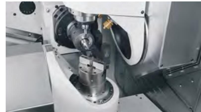
The swivel head axis is aligned with the tool centre point for maximum accuracy during simultaneous machining (Eliminating the need for compensatory movement in the milling axis).
