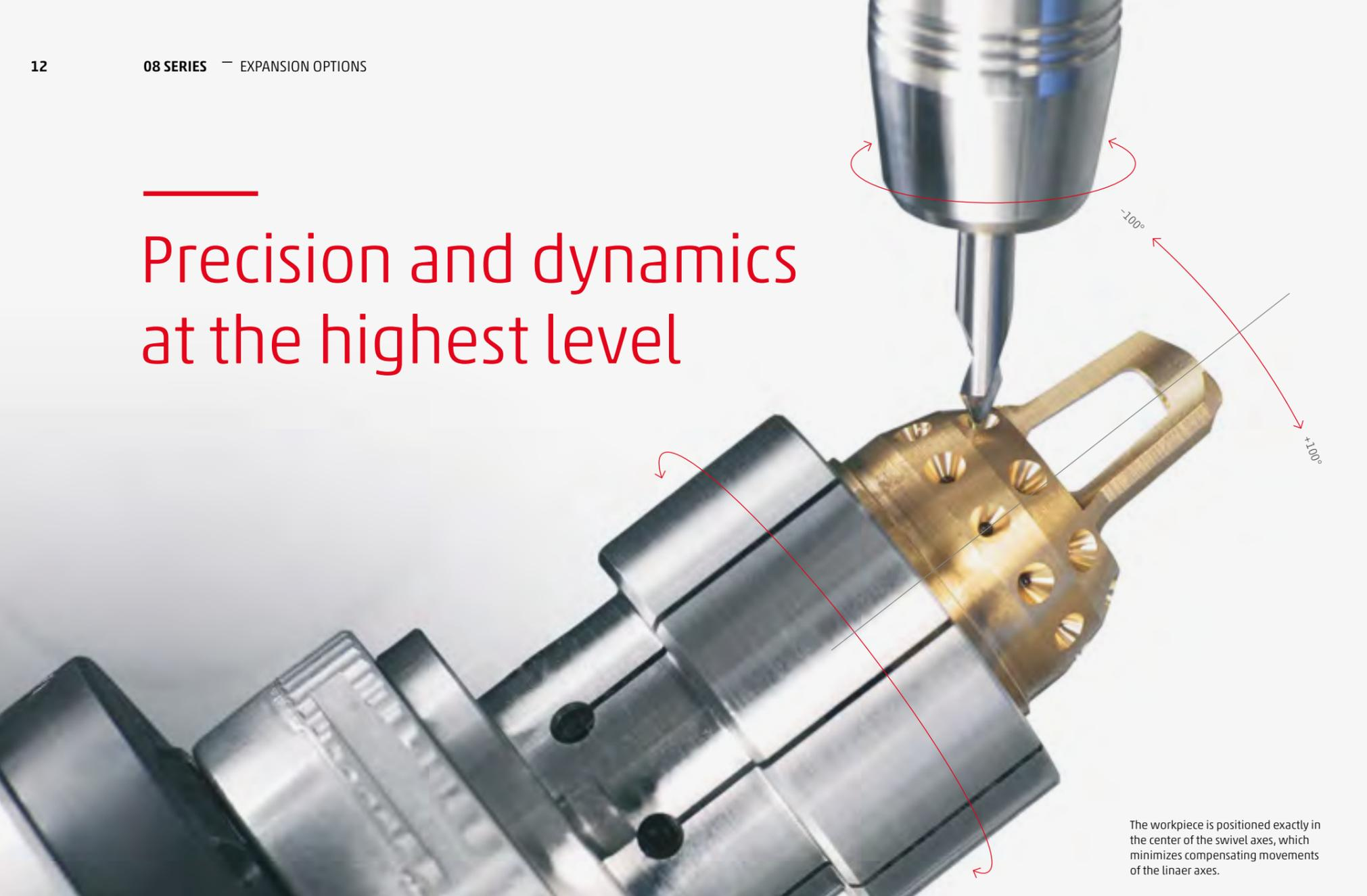
The workpiece is positioned exactly in the center of the swivel axes, which minimizes compensating movements of the linear axes.
