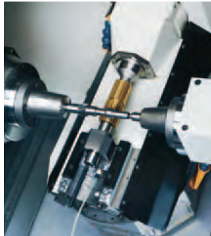
Machining area with hobbing head (direct drive)
