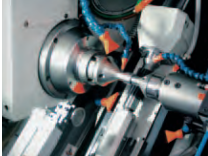
High-speed dry hobbing of planetary gears
