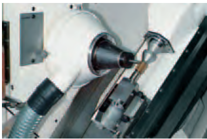
High-speed dry gear cutting of armature shafts
