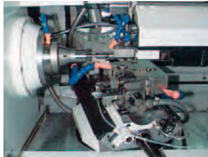
Angular milling head used as adaptor for shifting milling heads when milling single- and multi-start worms
