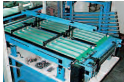
Long-time recirculating storage conveyor
