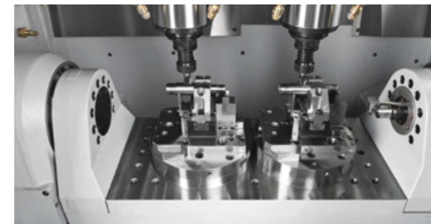
DZ 12 S five axis: Doubled productivity with minimal space requirements: fast double-spindle machining center with a 2-axis swivel rotary table (AC-kinematics) for efficient complete machining with five simultaneously controlled axes.
