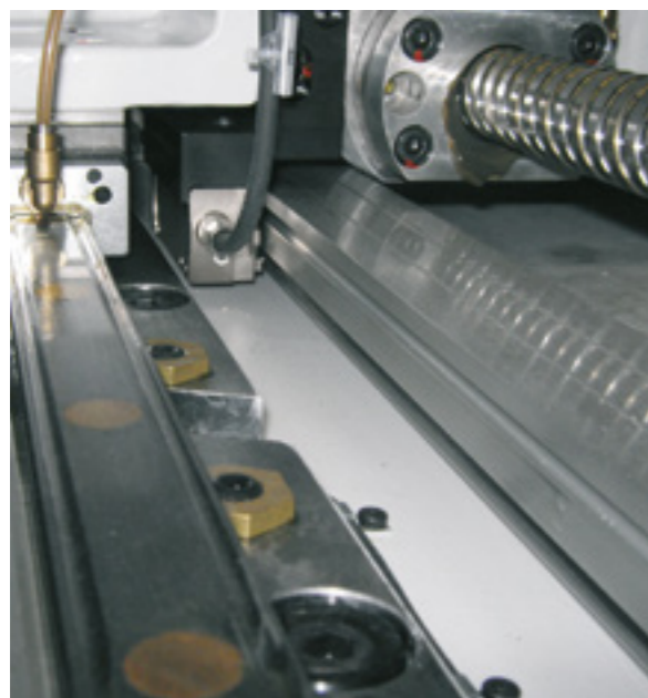
Highest precision: Glass scales and digital drive technology allow high acceleration with equally high contour accuracy.
