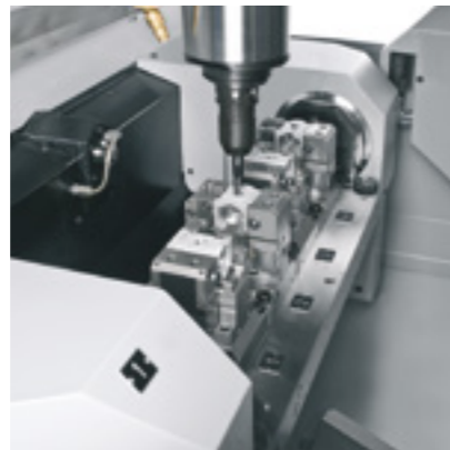
FZ 12 W Machining center with automatic tool change using the pick-up method and tool changing device for loading and unloading during machining
