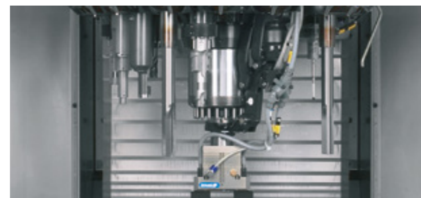
Workpiece gripper in the main spindle for machine-integrated workpiece handling.
