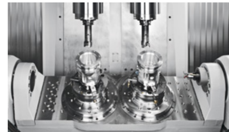
DZ 15 S five axis: Doubled productivity with minimal space requirements: fast double-spindle machining center with a 2-axis swivel rotary table with two face plates for efficient complete machining with five simultaneously controlled axes.
