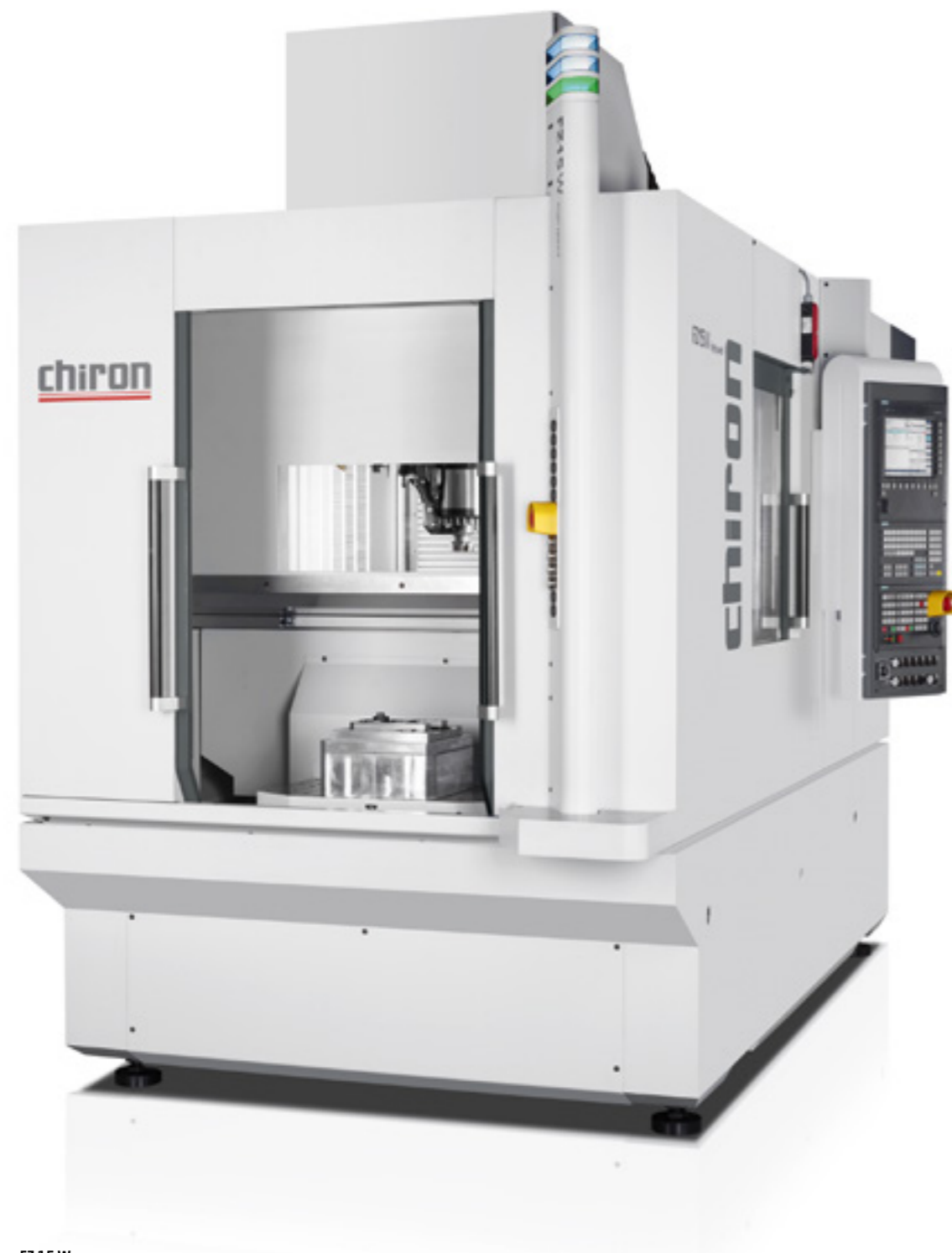
FZ 15 W Machining center with basket tool changer (20 tool) and workpiece changing device 0° / 180° enabling loading and unloading during machining.
