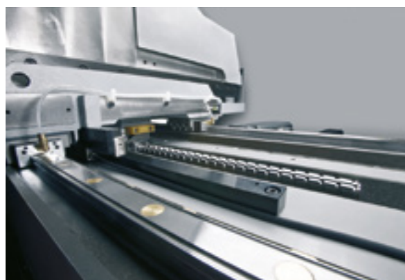
Highest precision: Glass scales and digital drive technology allow high acceleration and contour accuracy.
