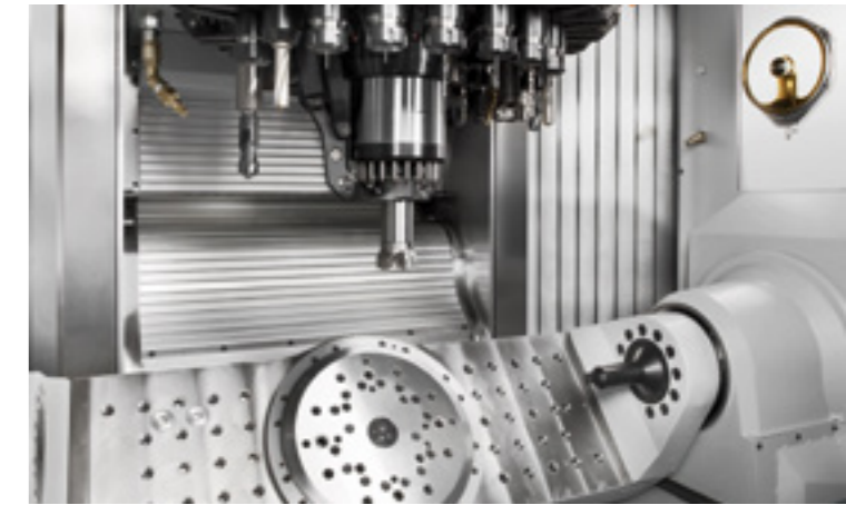
FZ 15 S five axis: Fast precision machining center with the fast CHIRON basket tool changer and a 2-axis swivel rotary table. High productivity, with chip-to-chip times as short as 1.7 seconds and tool changing times from 3.5 seconds.
