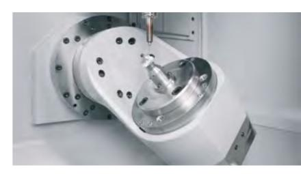
**FZ 08 S five axis:** Integrated 2-axis rotary table (BC kinematics), maintenancefree torque drive technology and automatic tool change with the pick-up method.
