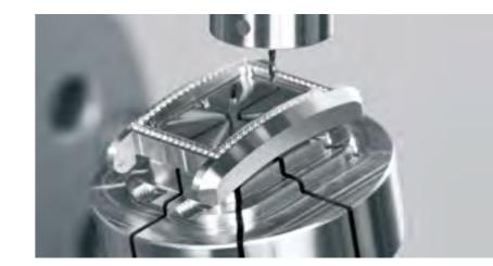
With the **CHIRON five axis** you achieve shiny surfaces, extremely fine structures, the smallest bore holes, grooves, pockets, fits and geometries with tolerances of a few microns – reliably, quickly and economically.
