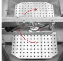
Workpiece changing device 0° / 180° with ample space for devices and NC rotary tables, such as the installation of a workpiece swivel device as the fourth
