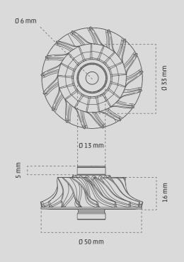
**Automotive**Compressor wheel for turbochargers
