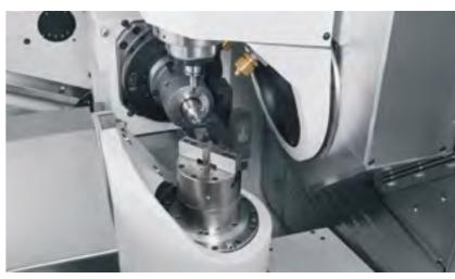
The swivel head axis is aligned with the tool centre point for maximum accuracy during simultaneous machining (Eliminating the need for compensatory movement in the milling axis).
