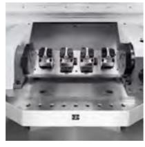
Perfect combination of two spindles, workpiece changing device 0° / 180° and NC rotary table with 4-way clamping device for multi-sided machining.
