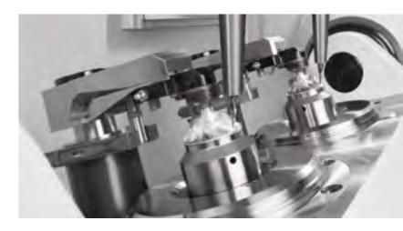
**DZ 08 S five axis:** Double productivity in a small space. The smallest and fastest double-spindle machining center with a 2-axis tilt rotary table (AC-kinematics) for efficient complete machining with five simultaneously controlled axes.
